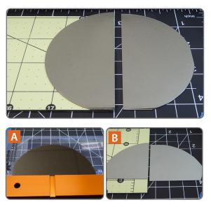
Figure 2, 2A & 2B. This shows the placement of the 4" wafer. After gently pressing the edge of the GaAs wafer, the cleave naturally occurs.
